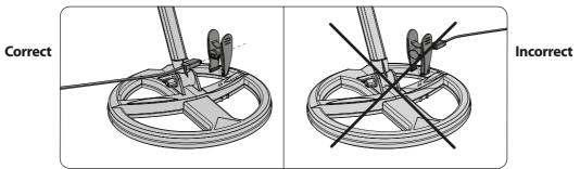
Ensure that the clamp is the right way round before connecting it to the coil
