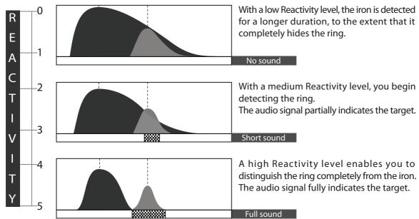
In terms of pure performance, the greatest detection ranges are obtained with low reactivity levels. However, you will find more targets on difficult ground with medium or high reactivity levels.
