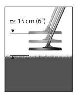
Pumping is a semi-automatic process which allows you to adjust the ground balance in a zone that you have determined as being representative of the mean level of the ground being prospected.
