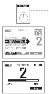
1 Press MENU 2 Scroll with and select REACTIVITY 3 Press EXPERT 4 Adjust the Silencer with | (-)(+) 5 Press x2 to return to the main menu.
